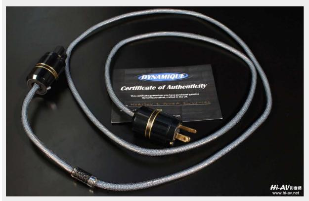
The thinner entry-level Horizon 2 power cord is limited by cost and cannot use sterling silver conductors, but the internal 6 strands of 19 AWG solid 7N oxygen-free copper wires and 1 strand of 16 AWG solid 7N oxygen-free copper ground wires are all silver-plated to make the high-frequency extension conduction smoother through the skin effect.
